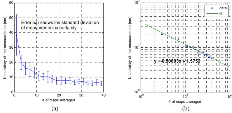
Fig.2. Measurement noise as a function of measurements averaged (a) normal scale (b) log scale
