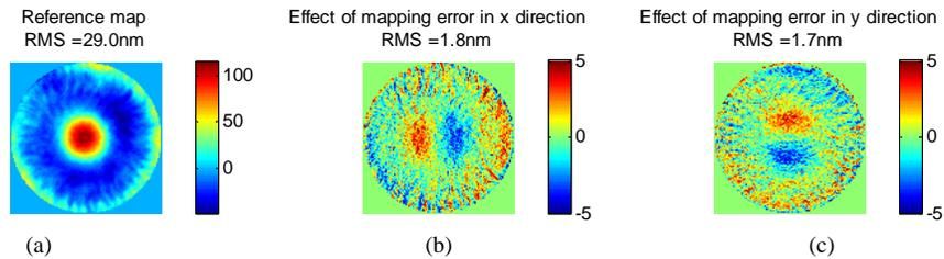
Fig.3. Reference map (a); Wavefront error due to 2-pixel mapping error in x direction (b); Wavefront error due to 2-pixel mapping error in y direction (c)
