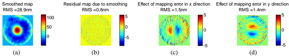
Fig.4. Smoothed reference map with a 7X7 filter (a) Residual small-scale error after smoothing (b) Wavefront error due to 2-pixel mapping error in x direction (c); Wavefront error due to 2-pixel mapping error in y direction (d)
