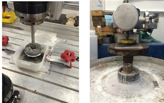
Fig. 1. The two setups used to grind and polish the ceramic sample. (Left) Initial work with a CNC machine. (Right) Final polishing with a Strasbaugh machine.
