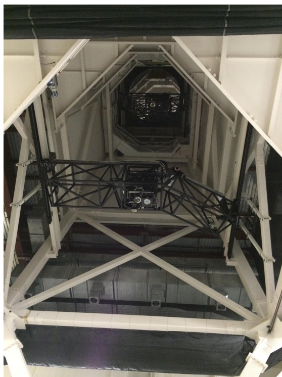
Figure 4. View of LSST test optics looking up into test tower from edge of mirror. Lower (closer) bridge contains M3 null test and upper bridge contains M1 test.
