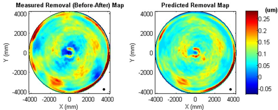
Fig. 3. Comparison between the measured and predicted removal map for a figuring run targeting mid-spatial frequency errors on the 8.4m GMT primary segment. The 250mm diameter RC lap used for the run is depicted in scale as a black disk at the bottom-right corner. (Note: Red areas (higher value) mean more removal.)
