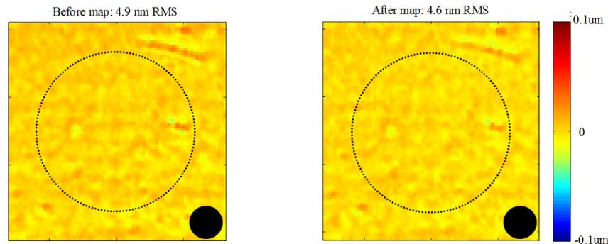
Fig. 4. Comparison between the before and after surface maps for a 40 hour smoothing run using a 1200mm stressed lap with pitch. The maps are high-pass filtered with  $0.0067\text{mm}^{-1}$  cut-off frequency, and zoomed in to  $\sim 1.7 \times 1.7\text{m}$  area on the 8.4m GMT primary segment.
