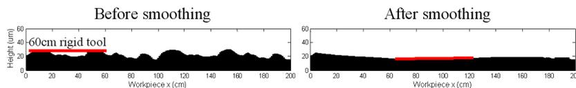
Fig. 1. Smoothing simulation for an infinitely rigid tool [10]
