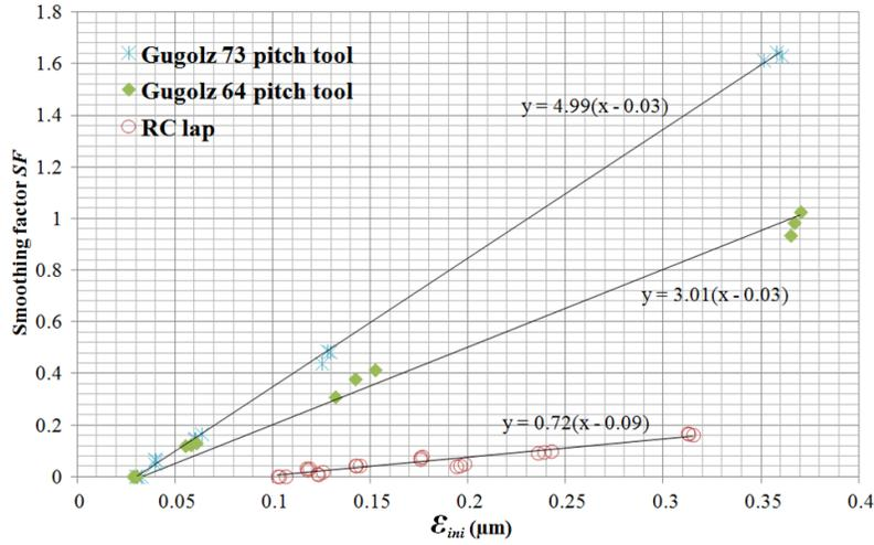
Fig. 2. Measured smoothing factor  $SF$  for two rigid tools using different pitch types and a Rigid Conformal lap with polyurethane polishing pad. [10]
