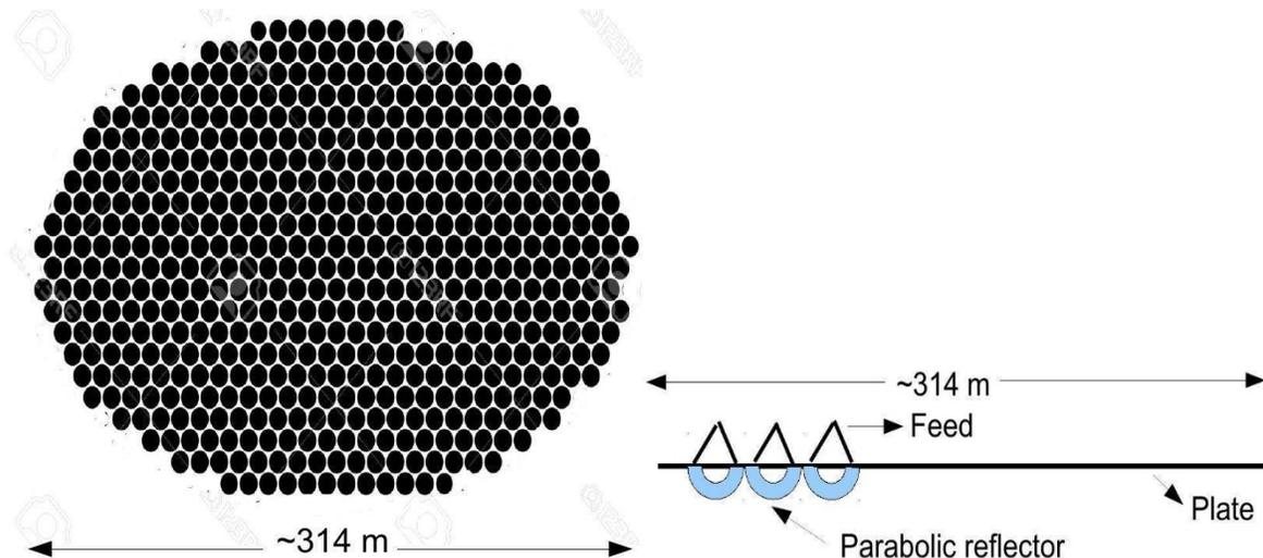
Fig. 1. A schematic of the NGAT concept showing an array of smaller dishes (left) and a cross section showing dishes co-mounted on a steerable platform (right). Image credit Arecibo Observatory.
