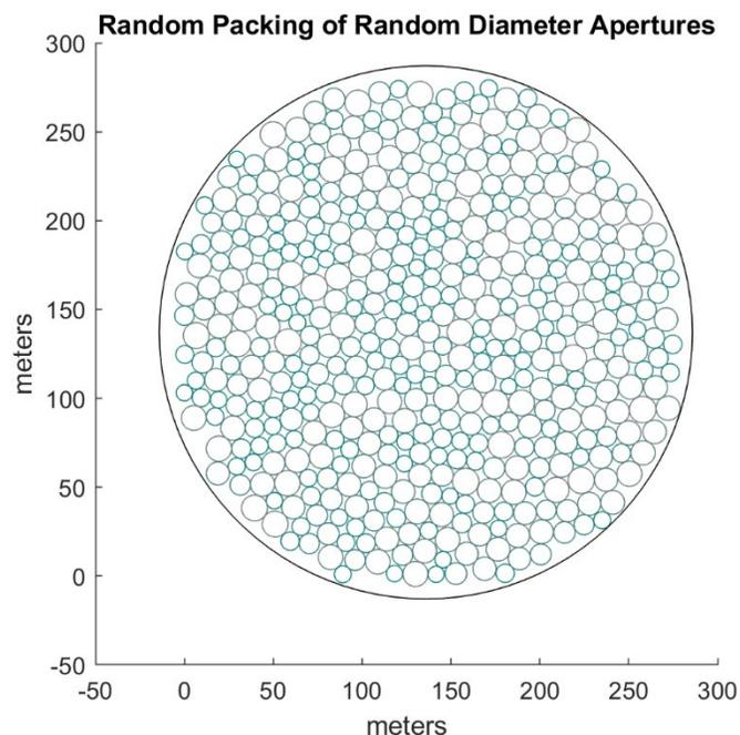
Fig. 2. A schematic of an array configuration that uses dishes with random diameters (flat distribution) ranging from 9 to 15 m in diameter that are close packed within a 300 m diameter circle.
