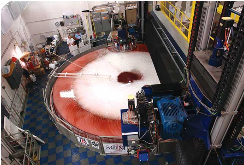
An 8.4-m primary off-axis segment mirror for the Giant Magellan Telescope being fabricated using a stressed lap at the Richard F. Caris Mirror Lab, Steward Observatory, University of Arizona. Courtesy of Steward Observatory, University of Arizona.
