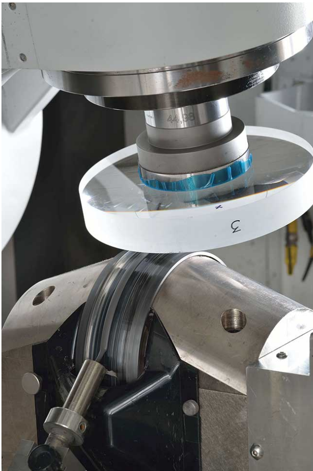
Deterministic polishing of a large aperture lens using magnetorheological finishing. Courtesy of QED Technologies Inc.
