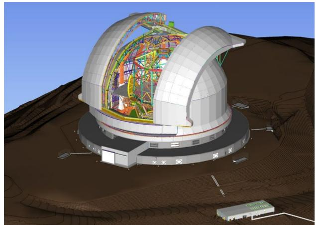
**Fig. 29** The E-ELT enclosure will be a super-massive structure which houses the 40-m telescope. The structure currently is designed as a hemispherical dome with two sliding doors that will open the telescope to the night skies. The entire dome rests on a circular track which will allow for rotation of the enclosure. Due to the enormous size, multiple support structures are planned to maintain the required stiffness and positioning accuracy of all components [83]
