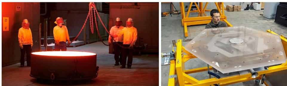
**Fig. 12** The E-ELT primary mirror uses a multi-step process to generate the final mirror segments. Initially, a circular mirror blank is fabricated and sent for further processing (left). The circular mirror segments undergo grinding, and rough polishing. The mirror support
