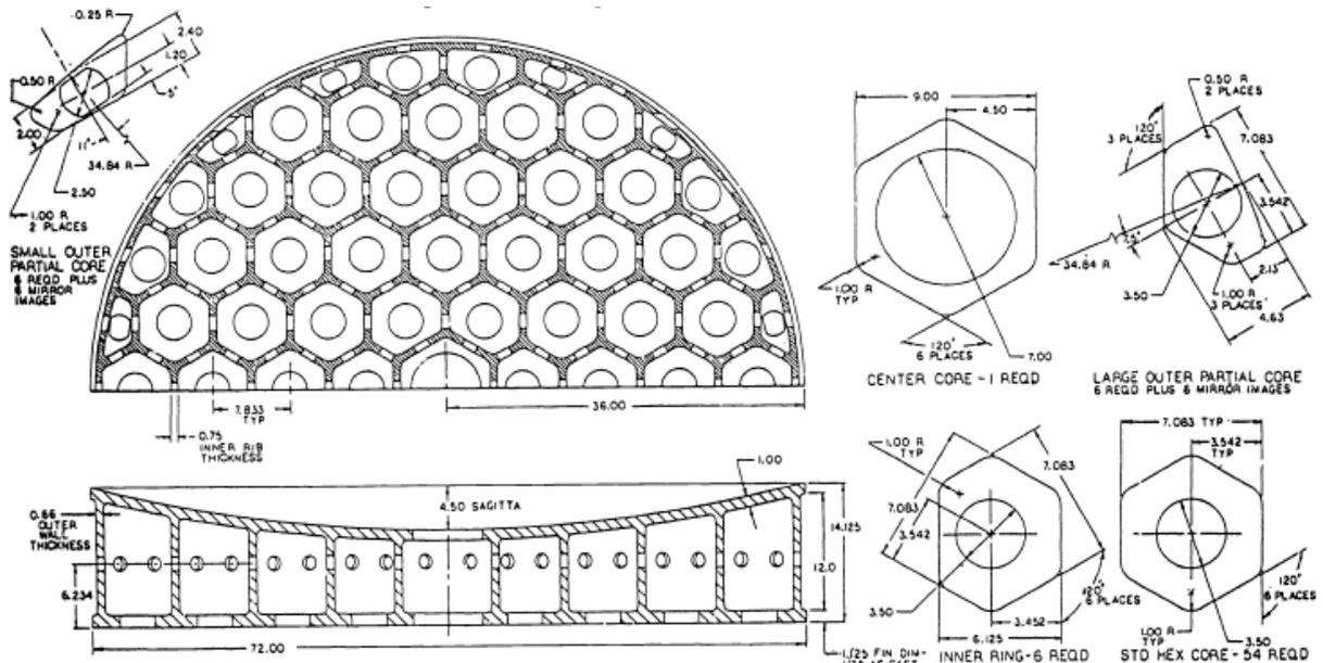
Fig. 1. Dimensions in inches of the first spin-cast mirror at the University of Arizona.
