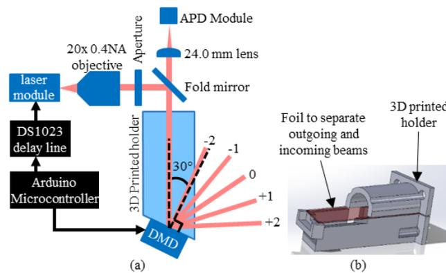
Fig. 2. (a) depiction of the physical LIDAR setup and (b) a depiction of the 3D printed mount.
