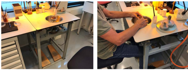
Fig. 1. Foot-driven polishing machine at an optics shop in Delft, The Netherlands.
