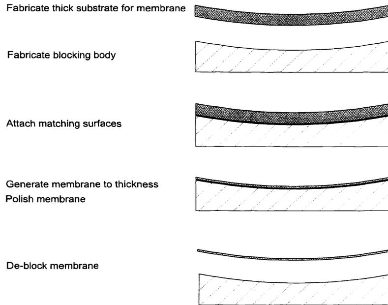
Figure 7. Concept for fabricating thin glass membranes.
