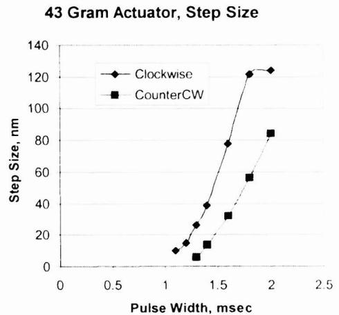
Figure 22. Measured motion of the prototype actuator. By adjusting the width of the pulse feeding the solenoid, the size of the step can be adjusted from a few nanometers to 0.1  $\mu\text{m}$ .
