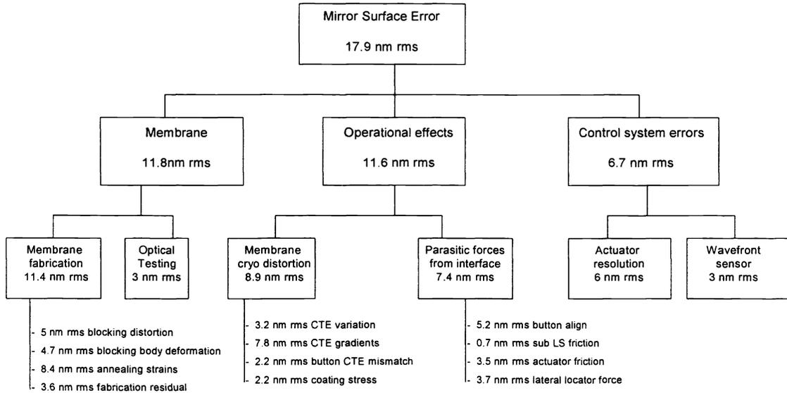
**Figure 3.** Error budget for the 2-m NMSD for operation at at 35 K.
