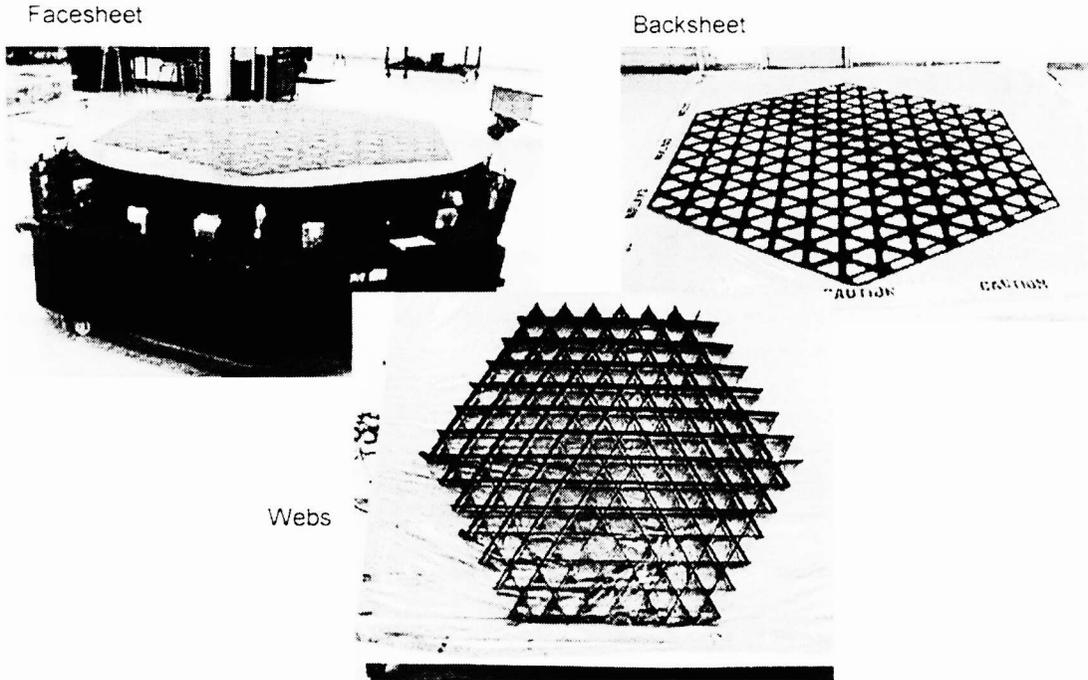
Figure 18. Components for the composite support structure at COI
