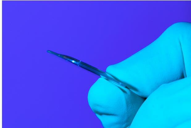
**Fig. 1** Prototype MODE lens fabricated at The University of Arizona. Although only 2–5 mm thick, MODE lenses combine two diffractive and one refractive optical element. In essence, they are ultralight, high-performance, three-element-integrated lenses that can be cost-effectively replicated.
