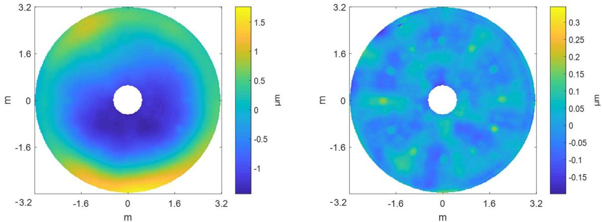
Figure 5. The difference between the final averaged surface error maps of the infrared deflectometry (including thermal bending correction) and null interferometry (including coma correction) having the RMS error of  $0.73 \mu\text{m}$  (left) and the residual of the difference map with 37 Zernike terms removed having an error of  $0.04 \mu\text{m}$  RMS (right).
