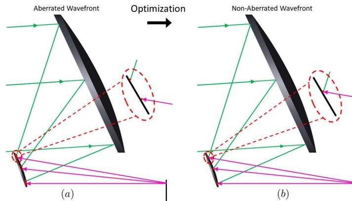
Figure 1. Forward (green) and reverse (magenta) ray data is used as the input to the parametric fitness function. As optimization converges to a local minimum, the aberrations in the system are reduced and the two data sets converge as shown in the call-out. [3, 4]
