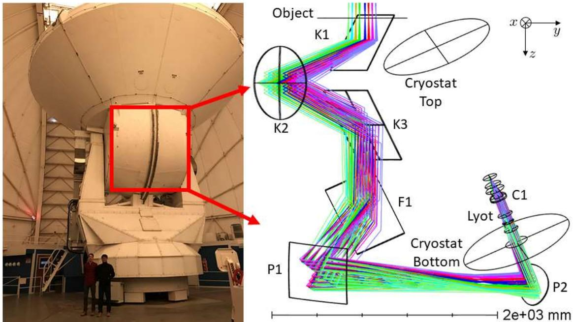
Figure 2. The 12-meter ALMA prototype radio telescope (left) on Kitt Peak in Arizona with its cabin called out, which houses the Tomographic Ionized-carbon Mapping Experiment (TIME) (right). The TIME optical design required an extremely folded beam path to fit the large linear FOV and cryostat in the defined volume of the telescope cabin. [3, 4]
