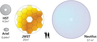
While this is not what the Nautilus mirrors will look like, this illustration shows the total collecting power of the fleet of 35 space telescopes. Each individual Nautilus mirror will, however, be able to collect more light than the Hubble Space Telescope. Credit: Nautilus team
