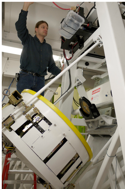
Figure 6: The small fold sphere attached to the test tower is shown at right. The final polishing surface map (left) is 4 nm rms, and this increases to 15 nm rms when mounted in the Sam support cell.
