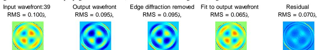
Fig. 4 Computer simulation of wavefront propagation for the standard Zernike term 39 with a Fresnel number of 50. The first column is the input Zernike functions with an error of  $0.1\lambda$  rms. The second column is the output wavefront after propagating a distance of  $L$  in a collimated space.
