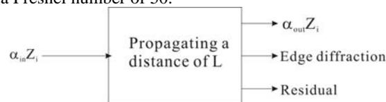
Fig. 3 As a Zernike term propagates a distance  $L$ , there will be smoothing effect, edge diffraction and some residual errors.
