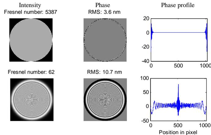
Fig. 2 Intensity pattern (left), corresponding phase pattern (middle) and the line cross-section along the diameter (right) due to edge diffraction at different Fresnel numbers. The wavelength is 632.8 nm.
