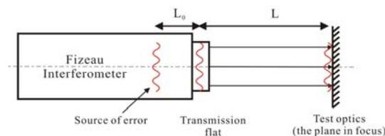
Fig. 1 A plane mirror, a distance  $L$  away from the transmission flat, is tested with a Fizeau interferometer.
