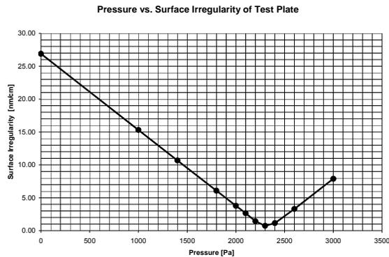
FIGURE 10. Pressure vs. Surface slope irregularity.
