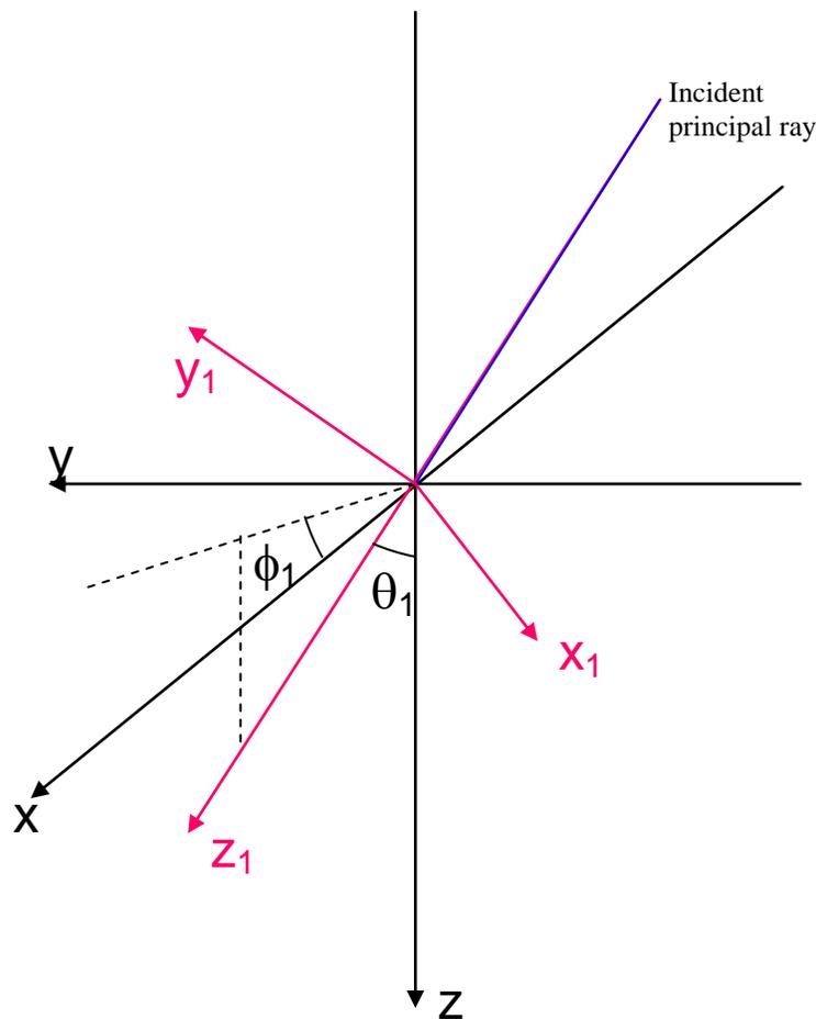
Figure 2. Illustration of coordinate systems' definitions for the refractive/reflective and diffractive surface and the incident wavefront:  $x$ - $y$ - $z$  is the coordinate for the surface and  $x_1$ - $y_1$ - $z_1$  is for the incident wavefront. The coordinate system for the refracted/reflected/diffracted wavefront is defined similarly as that of the incident wavefront.
