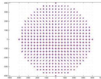
Figure 5. Illustration of the GMT null test system, and the locations and orientation of the astigmatic images of the test surface formed by the null optics.
