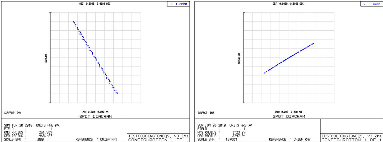
Figure 4. Explicit Zemax simulation showing the spot diagrams for image locations predicted by the generalized Coddington Equations to provide principal astigmatic focus.
