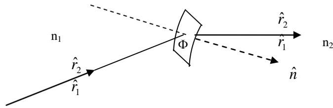
Figure 1. Illustration of a ray incident on a refractive and diffractive hybrid surface getting bent after the surface.
