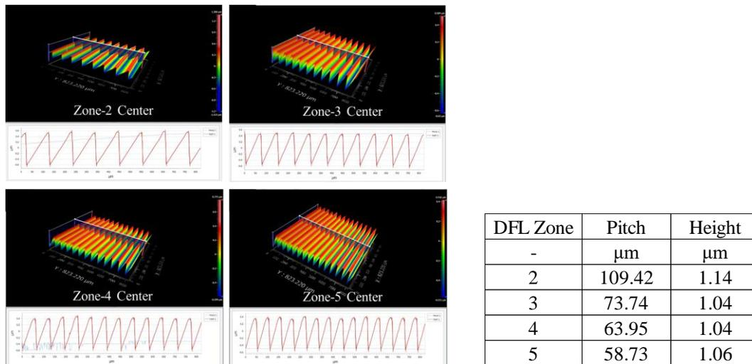
Figure 4. Single-harmonic DFL profiles measurement using Zygo NewView 3D optical surface profiler
