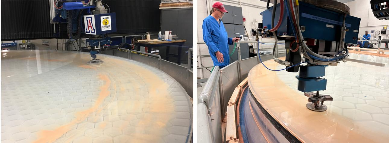
Figure 3. GMT Segment 3 being polished with a 40 cm pitch lap at left and a 10 cm lap at right. Both laps are driven by the same orbital polisher.
