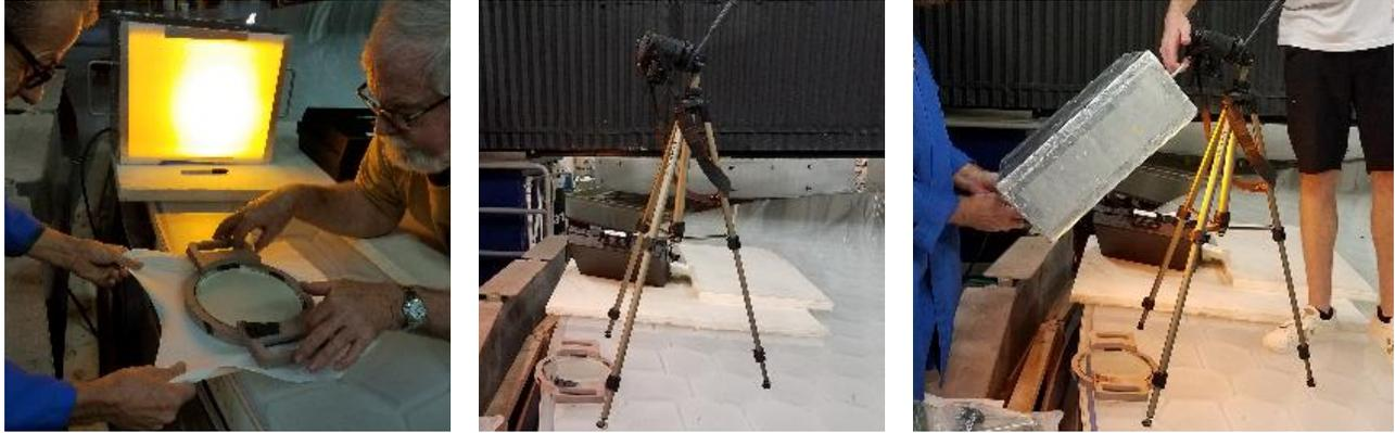
Figure 4. From left to right, the test plate is placed on the segment edge, the image used for alignment and scaling is taken under ambient light, and the fringe image is taken under a sodium light source with an average wavelength of 589 nm.
