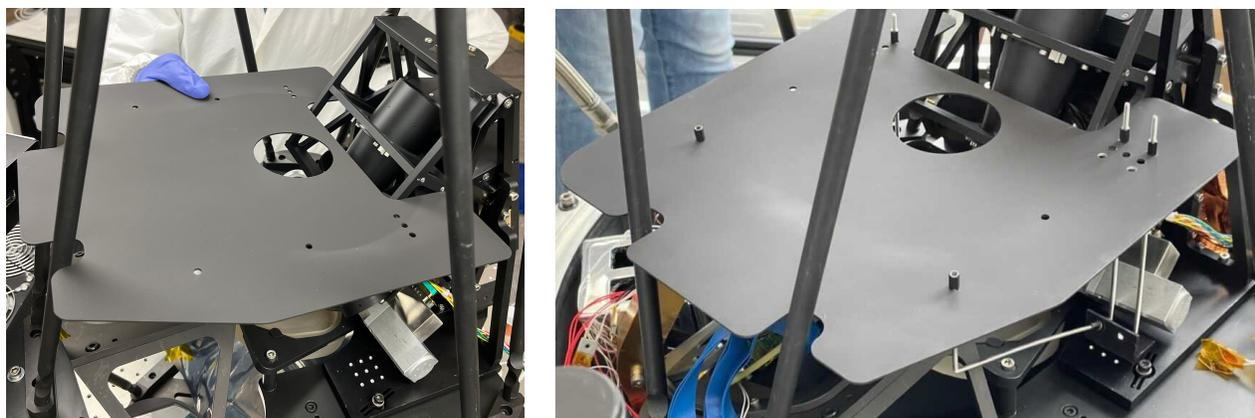
Figure 19. (Left) The pupil plane baffle positioned above the spectrograph medium bench during a fit check. (Right) The installed pupil plane baffle after detector shimming. Thin rods are used to hold the pupil plane baffle in place.
