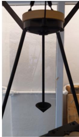
Figure 17. The conical baffle is fastened onto the FC1 mounting ring and sits beneath the field corrector assembly.
