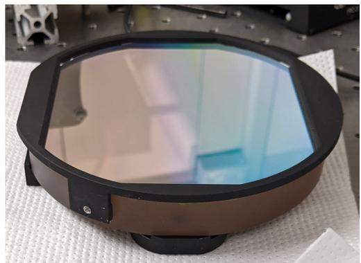
Figure 8. (Left) The grating mask with fixed to the outer face of the grating blank. Spacers shown in blue are used during mask installation to prevent damage to the grating surface and then removed after the adhesive sets. (Right) The coated grating mask during a fit check on the flight grating. The mounting mechanism was later updated as shown in § 6.6.
