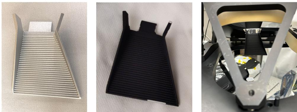
Figure 10. (Left) The tongue baffle upon receipt from ProtoLabs post manufacturing. (Center) The baffle was later coated with Avian-S optical black at Caltech to minimize scattering near the detector. (Right) The tongue baffle installed onto the FF2 mirror hole.
