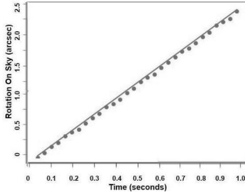
Figure 12. Rotation angle of slew bearing measured in successive video frames, taken at 30 frames/second.
