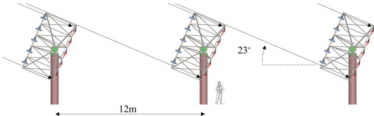
Figure 3. Telescope mounts at 12 m spacing, with unobstructed view down to  $23^\circ$  elevation
