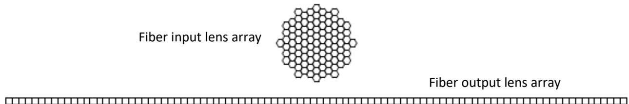
Figure 1. Upper, an array of 96 hexagonal lenses at the ELT  $f/20$  focus divides the light across a 1.11 arcsec aperture and directs it into 96 fibers. Lower, a line of 96 lenses of the same focal length, now cut into squares of the same area as the hexagons, directs the fiber outputs to form the  $f/20$  slit input to the spectrograph.
