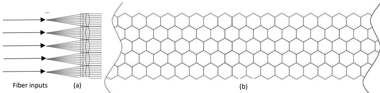
Figure 4. An array of 5 x 528 fibers and hexagonal lenses to combine the light into a single large-scale slit. (a) Side view (b) face-on view of a section of the array.
