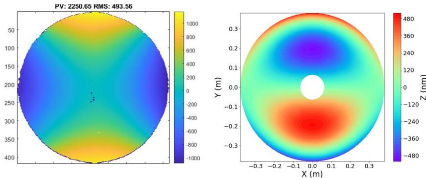
Figure 11 a) Astigmatism of  $2.2 \mu\text{m}$  P-V induced in the 200 mm BK7 test mirror, using only the 8 edge actuators, measured using phase shifting interferometry. Color scale in nm. Figure 11 b) ANSYS finite element model of coma induced in the 0.76 m Borofloat mirror assembly of Figure 9, using all 132 actuators.
