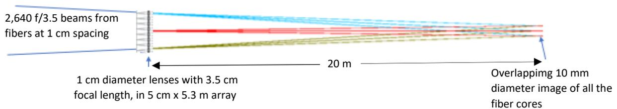
Figure 5. Schematic ray diagram, not to scale, showing how the images of the individual fiber cores formed by the hexagonal lens array overlap at a common exit pupil
