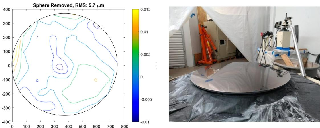
Figure 7. Left, departure from a sphere of a 0.76 m Borofloat disc slumped disc, slumped over the prototype spherically ground mandrel. The surface contours are at 5  $\mu\text{m}$  intervals, from CMM profilometry. Right, a second, more rigid and polished mandrel ready for slumping tests of 0.81 m substrates.
