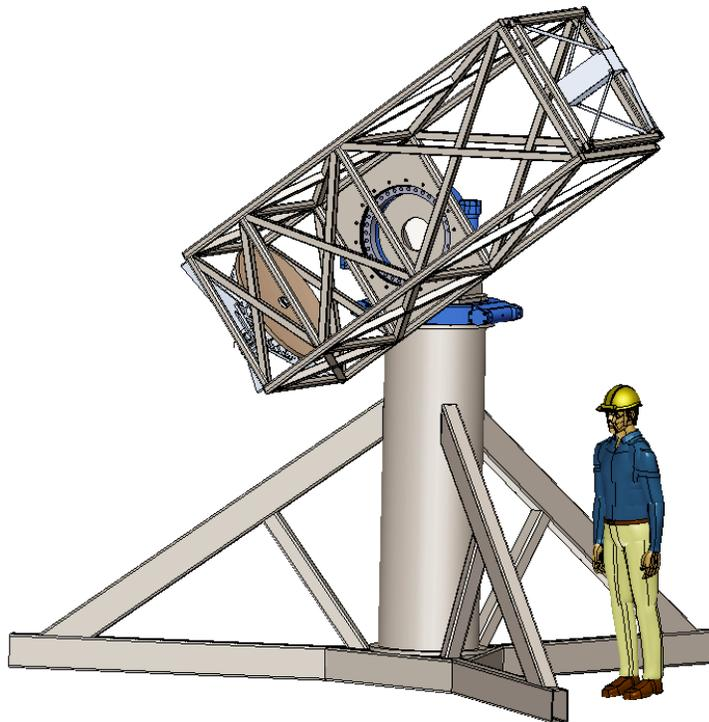
Figure 13. Single unit telescope prototype on an alt-az test mount
