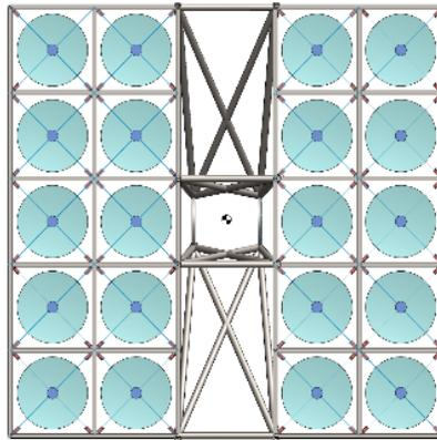
Figure 2. Plan view of mount with 20-unit telescopes
