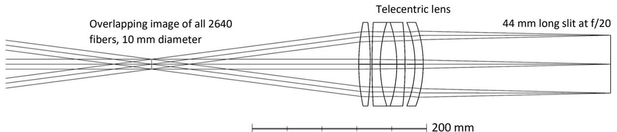
Figure 6. Telecentric lens at the common exit pupil, forming a 44 mm long slit at f/20 at the entrance to the spectrograph
