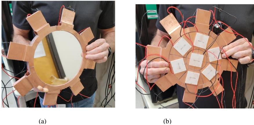
Figure 10. 200 mm test mirror with 15 Peltier thermal actuators. a) Front view, b) back view, prior to attachment of heat sinks on the 7 back actuators.
