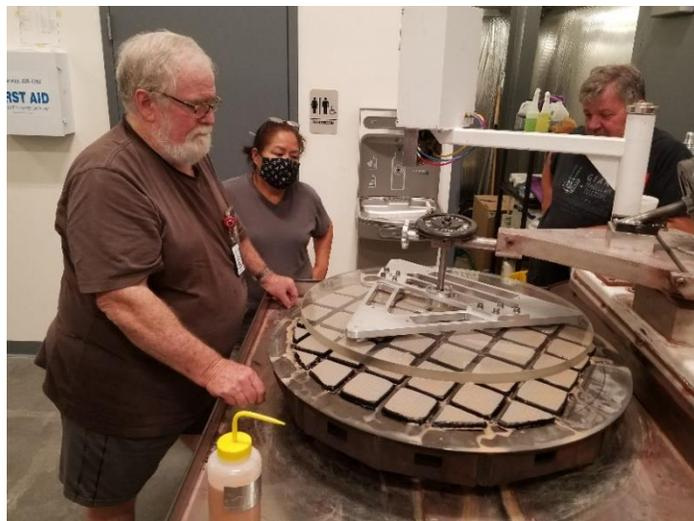
Figure 8. Optical finishing of the 30" slumped disc with a 36" polishing machine
