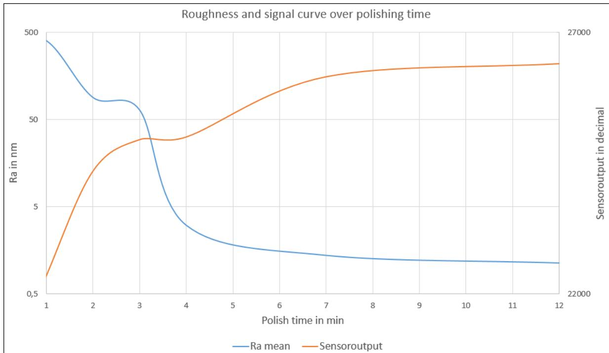
Fig. 3: Photo-optical sensor signal and the surface roughness evolution during the optical polishing process of the experimental sample workpiece surface area.
