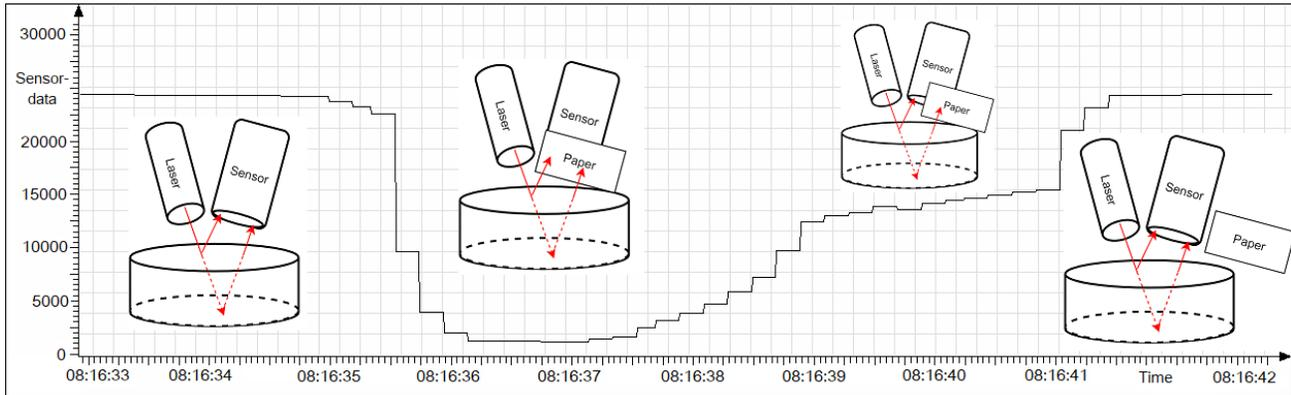
Fig. 2: Experimental validation of the two beam measurement data signal using a beam blocking mask in front of the photo-optical sensor aperture.
