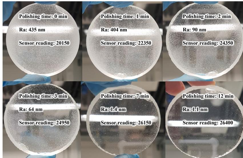
Fig. 4: Visual quality and the surface roughness (i.e., Ra) evolution of the experimental polishing sample surface during the polishing process until the surface roughness Ra value reaches about 1.1 nm.
