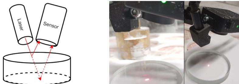
Fig. 1: Schematic measuring principle of the in-process surface roughness measuring device (left) and actual experimental hardware set up using the laser and photo-optical sensor (right)
