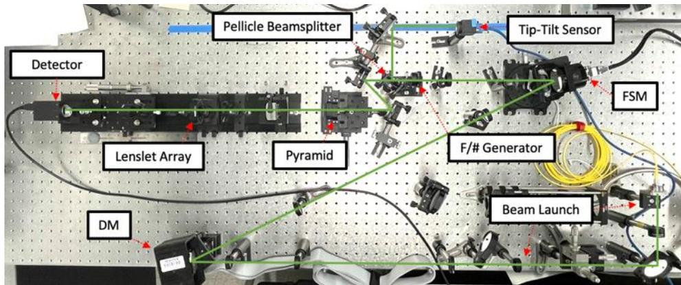
Figure 6. Labeled photograph of the actual HyWFS test bench configuration with the green ray representing a nominal beam propagation axis.
