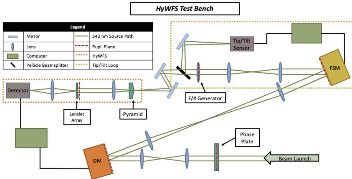
Figure 1. Schematic diagram of the HyWFS test bench configuration and beam path. The HyWFS is marked as the red-bordered box and the Tip-Tilt Loop is shown in the yellow-dotted box.
