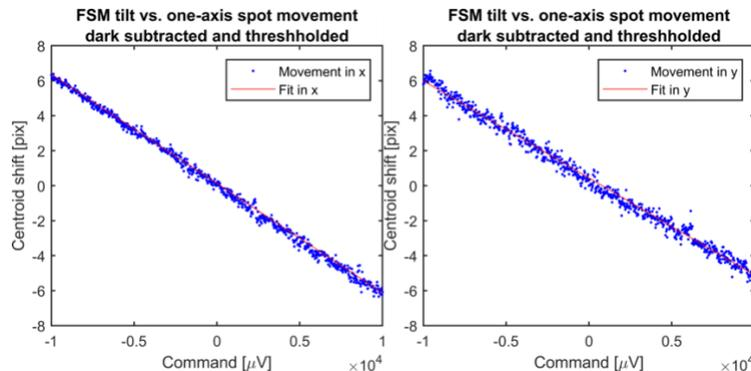
Figure 9. Spot movement, expressed as centroid shift in pixels, vs applied FSM command in  $\mu\text{V}$  when dark subtracted and thresholded images are used
