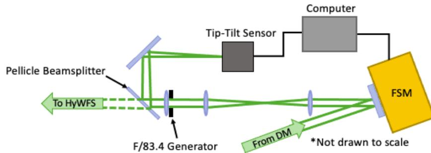
Figure 5. Schematic diagram of the TTL with the beam path shown at green rays. This corresponds to the components in the yellow-dotted box in Figure 1.
