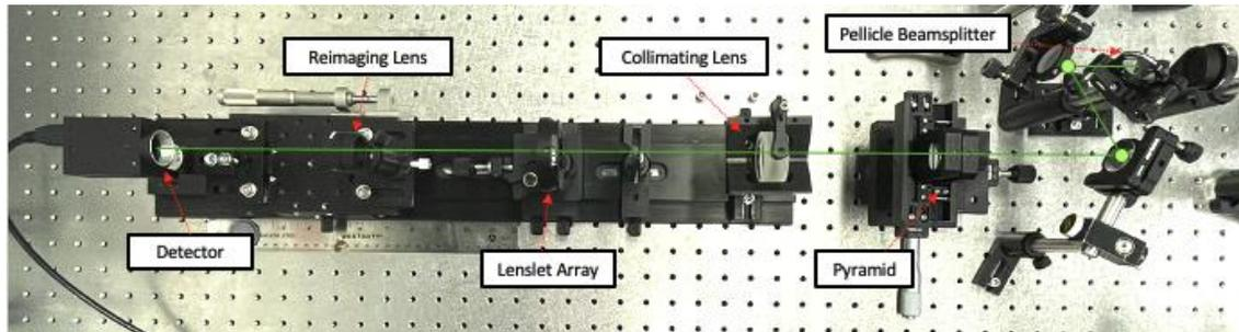
Figure 3. Labeled photograph of the HyWFS on the test bench, this corresponds to the components in the red-dotted box in Figure 1. The nominal beam propagation axis is shown as a green ray.
