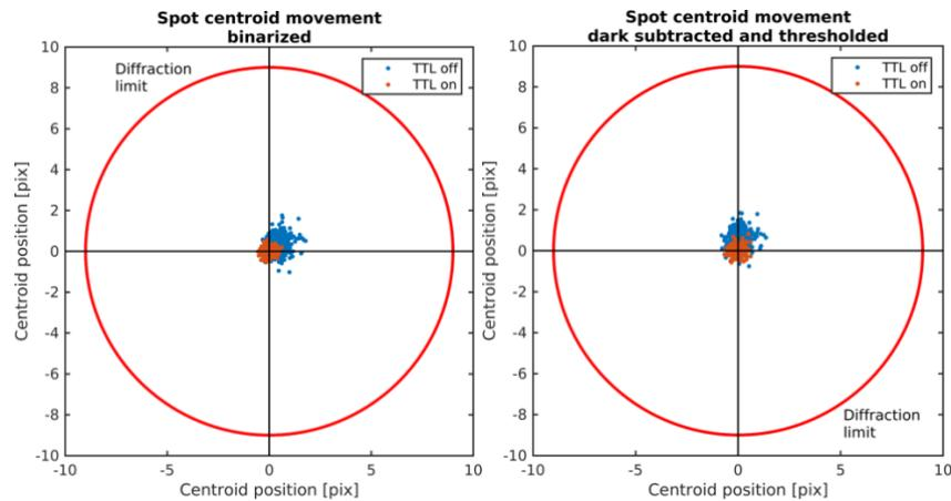
Figure 10. (left) Movements of focused spots, both with the TTL on and off, represented by 2D plot of centroid locations using binarization method. (right) Movements of focused spots, both with the TTL on and off, represented by 2D plot of centroid locations using dark subtraction and binarization method.
