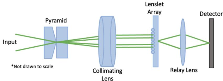
Figure 2. Simplified optical schematic of the HyWFS consisting of the pyramid prisms followed by the collimating lens to create the quadrant pupil plane at the lenslet array. The focused array of spots is imaged on the detector through the relay imaging optics.
