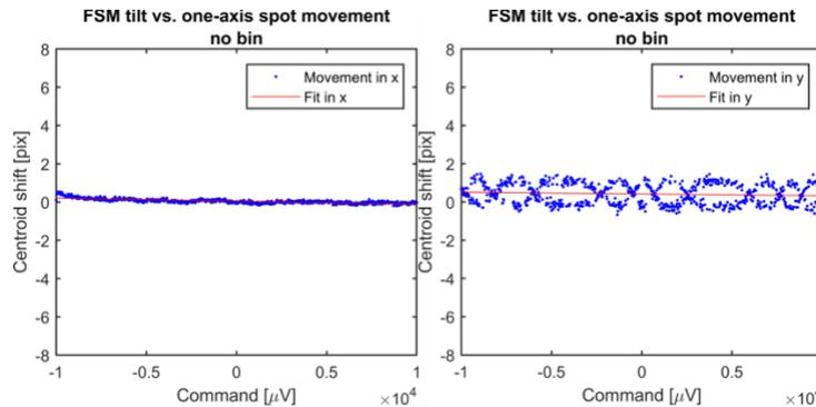
Figure 7. Spot movement, expressed as centroid shift in pixels, vs applied FSM command in  $\mu\text{V}$  when raw images are used
