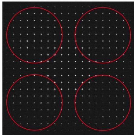
Figure 4. Measured irradiance image of HyWFS output at the final detector plane displaying the quadrant image of the focused spot array
