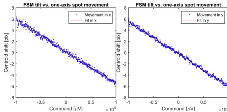
Figure 8. Spot movement, expressed as centroid shift in pixels, vs applied FSM command in  $\mu\text{V}$  when binarized images are used
