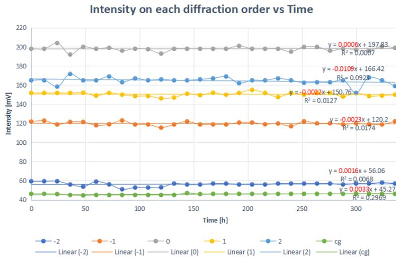
Figure 5. Results of continuously operating beam steering system under room temperature 25 degree C
