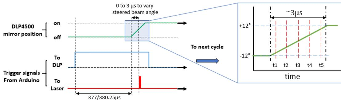
Figure 2. Timing diagram of DMD based diffractive beam steering with DLP4500. For global delay  $377\mu\text{s}$ ,  $t_1=0.5\mu\text{s}$ ;  $t_2=1.25\mu\text{s}$ ;  $t_3=1.875\mu\text{s}$ ;  $t_4=2.375\mu\text{s}$ ;  $t_5=2.75\mu\text{s}$ .
