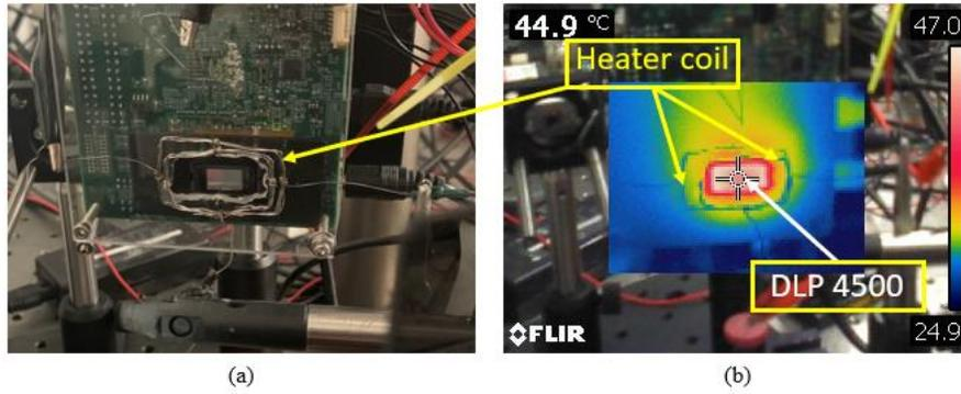
Figure 4. (a) Setup of heat cycling test. Heating coils are placed at the vicinity of DMD; (b) Temperature image captured by thermal imager
