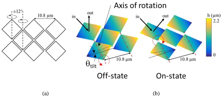
Figure 1. Representation of the (a) 0.45-inch DMD diamond pixel geometry (Top View) with  $10.8 \mu\text{m}$  pixel period, mirror can flip between  $\pm 12^\circ$ ; (b) Schematic of “on” and “off” state of micro mirrors
