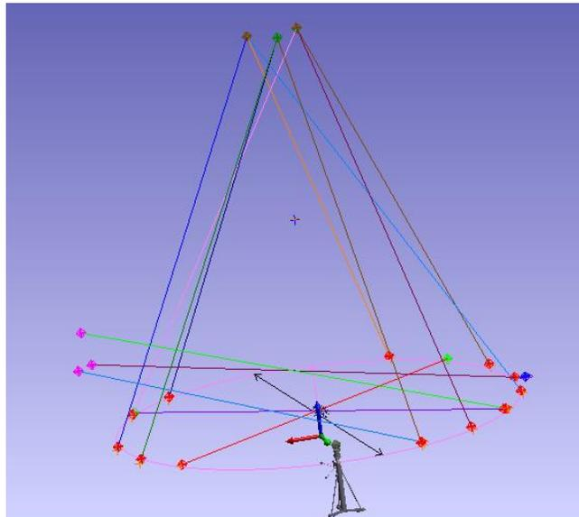
*Figure 1 Laser Tracker Survey of TMS launch collimator positions around the edge of the primary mirror on the Right hand LBT mirror (lower) and target points on the prime focus camera (upper three points). The survey is required to establish the base geometry for kinematics equations.*
