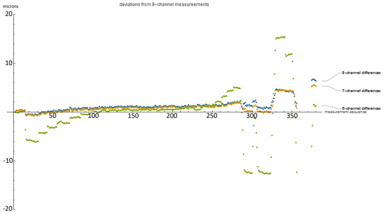
Figure 6. Investigating deviations in results between 8, 7 and 6 channel measurements we found clear degradation with reducing number of channels, but the errors were still less than 2% of commanded value at worst, with the 6-channel measurements. Note that the “large” 20 micron excursions at around measurement sequence number 300 occurred when the mirror was driven 1500 microns, so these differences are relatively small compared to commanded position.
