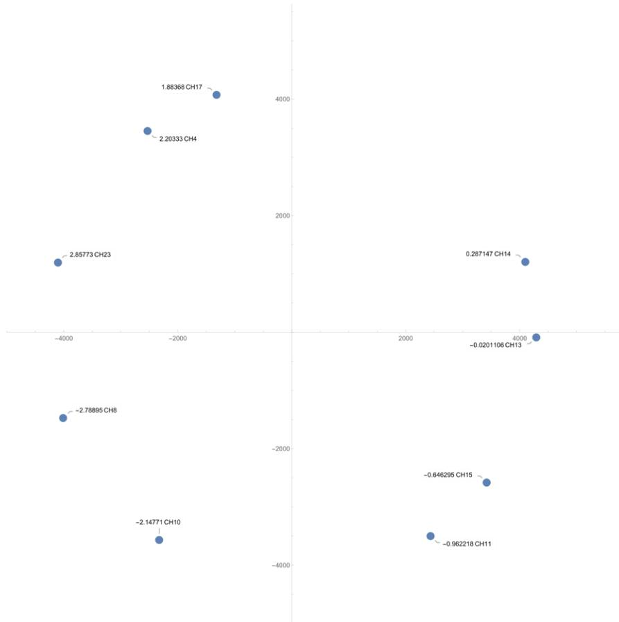
Figure 8. Azimuthal mapping of metrology channels for the current laser truss. Numerical values at each labeled channel are clocking angles in radians. The X- and Y-axes serve to indicate the position of each channel with respect to the center of the mirror surface in millimeters.
