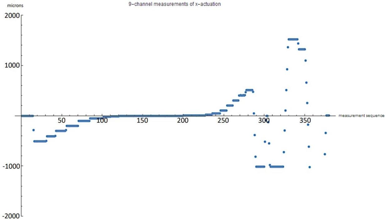
Figure 4. The primary mirror was sent to x-positions in the range of  $\pm 1.5$  mm, as the metrology truss measured position. In this case all nine channels were used. The vertical axis represents measured x-position of the mirror and the horizontal plot indicates time-sequential order of measurement. The greatest errors were less than 1% of the commanded position.
