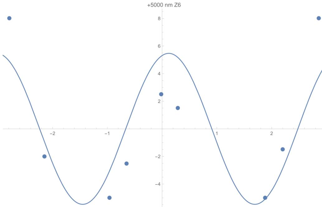
Figure 9. A representative fit of measured channel length changes back-projected to surface normal changes at various azimuth points, to an astigmatic shape change, as measured in the edge-zone of the mirror.
