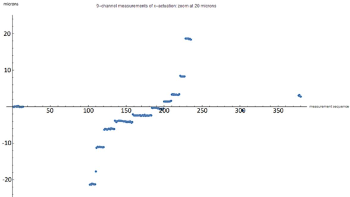
Figure 5. Zooming the y-scale from 2.5 mm to 25 microns shows the small-step resolution at a very reliable 2 microns. Each point is a single measurement at approximately a 7 second measurement interval. Looking at the point grouping the indication is that this is the actuator bit-resolution limit, not a measurement resolution limit.
