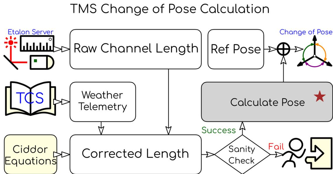
Figure 10. Overview of the major steps transforming raw TMS channel length to a preliminary correction vector (i.e., the “change of pose” vector). The shaded and starred box “Calculate Pose” is expanded and explained in detail in the text.
