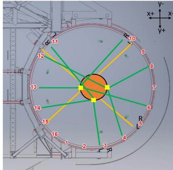
Figure 3. Channel paths connecting points indicated in Figure 1. In this table collimator launch points and retroreflector vertex positions are defined, and corresponding channels shown. The nine channels labeled “LBC” in Table 1 connect the outer disk (M1 edge) to inner disc (Prime focus camera) in this top-view schematic.
