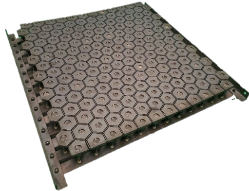
Figure 13. Adjustable mold: 50 x 50 cm prototype with bolts used as actuators adjusted from the back.
