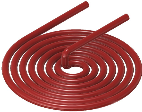
Figure 2. CAD drawing representing the coil used in the initial experiments with 7 turns made from a flexible cooper tube which cross section has 8 mm external diameter and 1 mm thickness, a 1 mm thick fiberglass jacket was used as electrical insulation.
