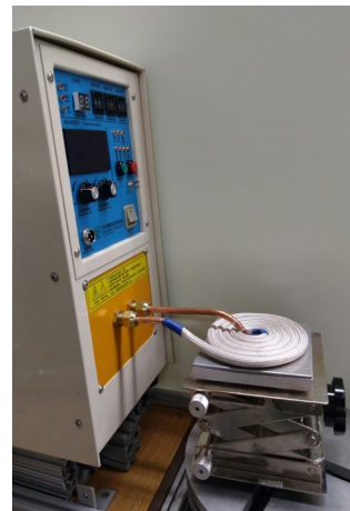
Figure 3. HT-15KW induction power supply with a small solenoid used in home ironwork process (left), pancake induction coil placed in the same power supply on top of the workpiece and ceramic mold (right).
