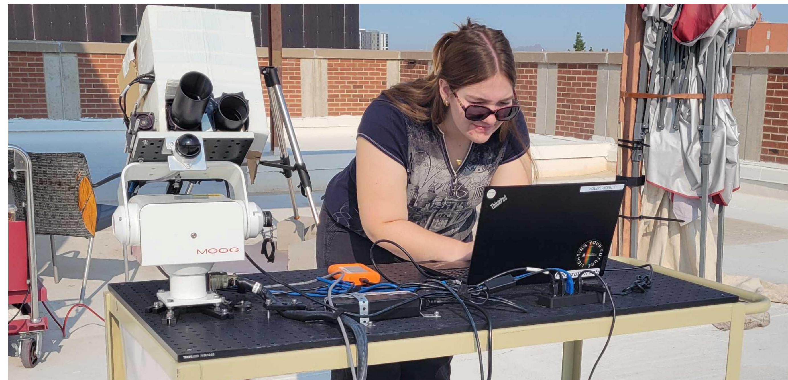
Fig. 2: ULTRASIP mounted on an altitude-azimuth motorized stage and cart for rooftop deployments
