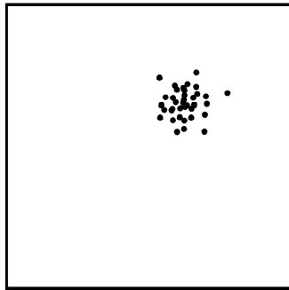
Fig. 12.28 Image of many gamma rays, all incident at the same position. As the number of gamma rays approaches infinity, this image approaches the conditional PDF \text{pr}(\mathbf{r}|\hat{\mathbf{r}}) .
