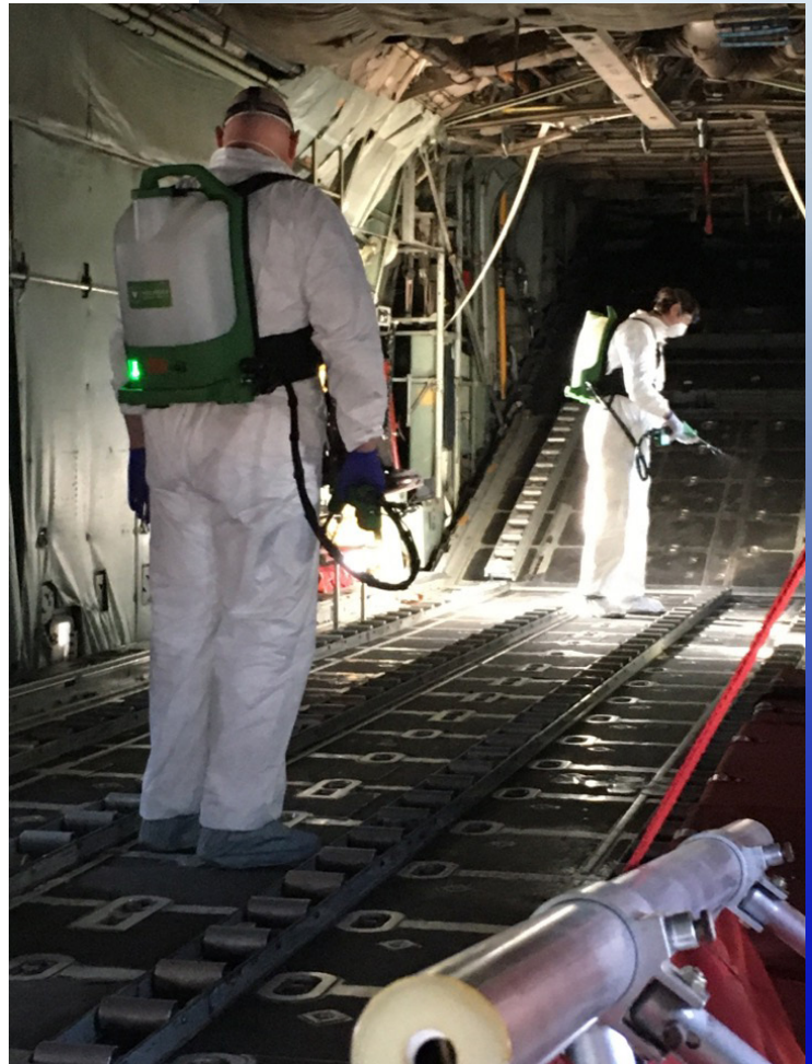
NSWC-DD researchers apply germinant solution to the interior of a C-130 aircraft during a field test at Holloman Air Force Base, NM. (Heather Welch/ Joint Research & Development, Inc. photo)
