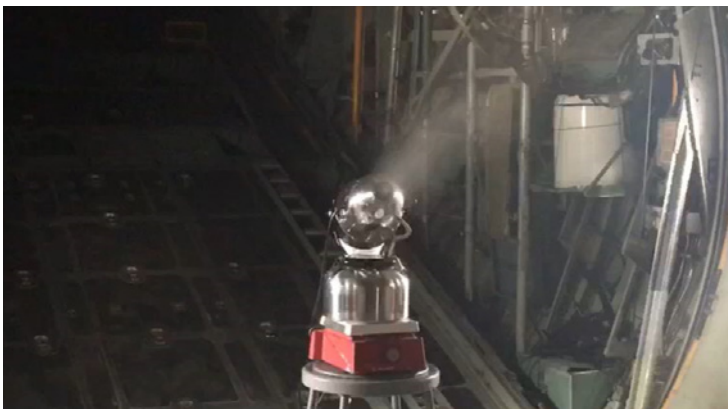
Fogging machines disseminated 100 million surrogate bacterial spores per square meter on the C-130 interior. (Heather Welch/Joint Research & Development, Inc. photo)
