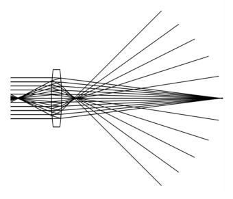
A singlet lens can have a single two-bounce ghost, a two lens system can have six, two-bounce ghosts, a three lens system can have 15 two-bounce ghosts, and the number of two-bounce ghosts increases as
