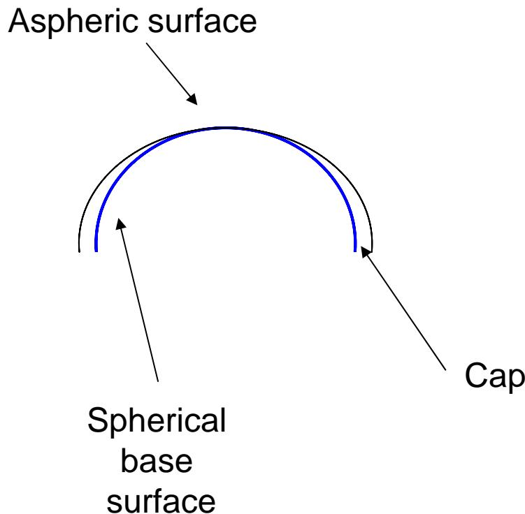
The aspheric surface can be thought of as comprising a base sphere and an aspheric cap
