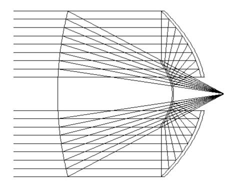
Since the equivalent refracting surface in a Cassegrain telescope is a paraboloid then the coma of that Cassegrain is the same of a paraboloid mirror with the same focal length.
