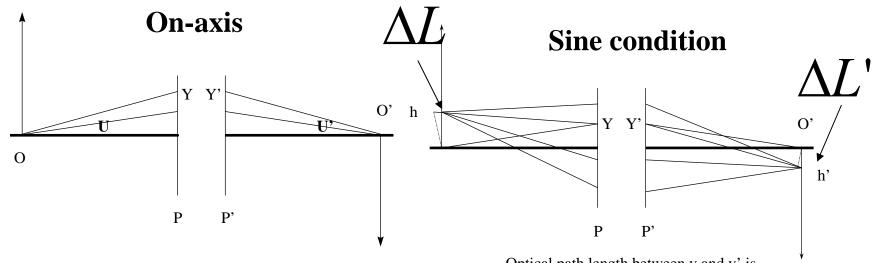
Optical path length between O and O' is  $L_{axis}$  and does not depend on Y or Y'
