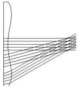
In the presence of a strong aspheric surface near the stop or pupil, coma aberration can be corrected by moving the surface
