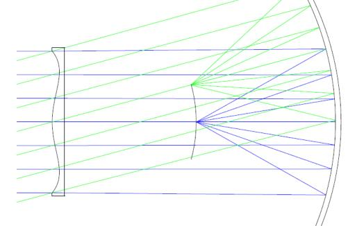
Aspheric plate at mirror center of curvature A-bar=0
