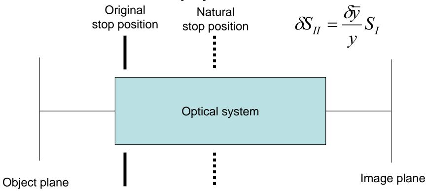
In the presence of spherical aberration there is a stop position for which coma is zero. At that stop position spherical aberration might be corrected. Then the system becomes aplanatic and the stop can be shifted back to its original position.
