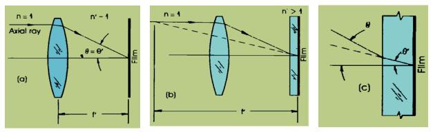
Figure 1. Posterior focal length for an image in air, and in a thin glass plate.
