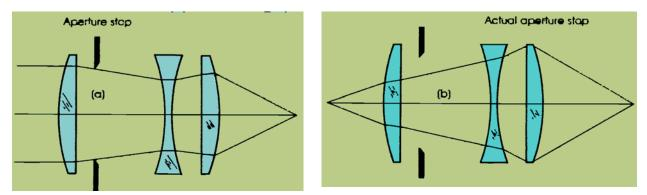
**Figure 2.** The effective aperture stop of an optical system can change when the system is used with a long conjugate (a) and a short conjugate (b).
