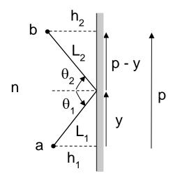
$$\frac{dOPL}{dy} = n\frac{dL_1}{dy} + n\frac{dL_2}{dy} = 0 \quad \text{for a valid ray path}$$
