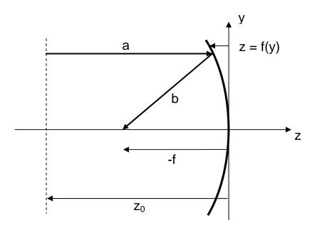
$z_0$  represents an arbitrary reference plane and is negative as shown. The surface sag z is also negative.
