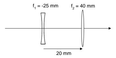
An object is placed 300 mm to the left of the first lens. The object size is  $\pm 10$  mm. Use paraxial raytrace methods to determine the system focal length and the location and size of the image.
