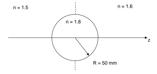
An object of size  $\pm 10$  mm is placed 500 mm to the left of the front vertex of the sphere.
