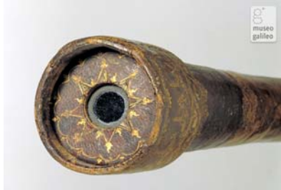
This 21X telescope from 1609-10 has a plano-convex objective lens with diameter of 37 mm, an aperture of 15 mm, and a focal length of 980 mm. The telescope is 927 mm long with a field of view of 15 arc min.
