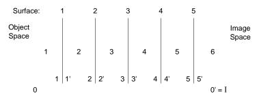
A single object or image exists in each space. Each surface has an object space and image space of its own. These intermediate optical spaces serve as the image space for the preceding surface and the object space for the following surface. Each surface will form an image of the object in the preceding space.
