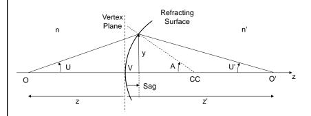
Approximation #3: The object and image distances are much greater than the sag of the surface at the ray intersection.
