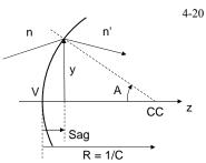
Approximation #2 implies that the sag of the surface at the ray intersection is much less than the radius of curvature of the surface.
