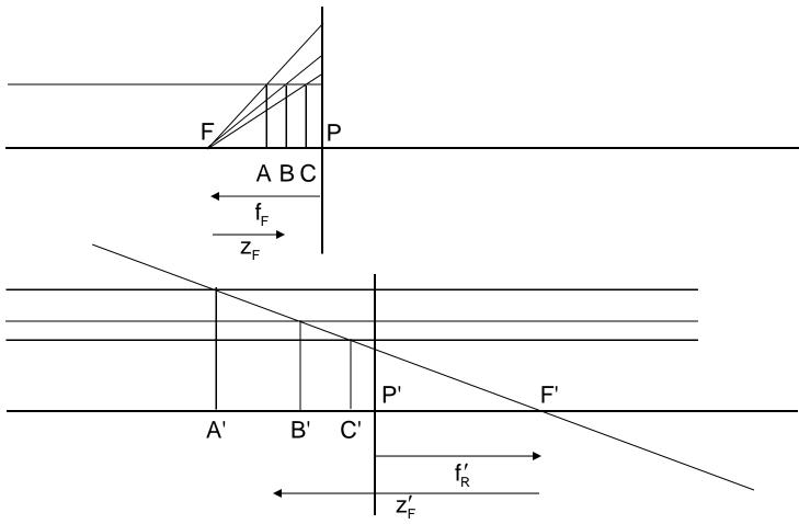
Images are erect and magnified Objects and images are in the same order  $z_F > -f_F$   $f_F < 0$  m > 0 (0 < m < 1)  $\Delta z' > 0$   $f_R' > 0$   $z_F' < 0$   $(-f_R' < z_F' < 0)$   $\Delta z' > 0$
