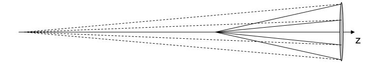
When the object goes to infinity, the rays become parallel or collimated.
