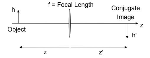
Because of sign conventions, an object to the left of the lens has a negative object distance.
