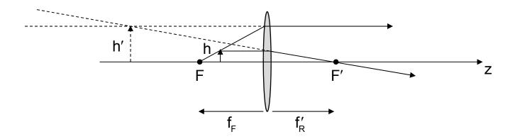
The two image rays diverge and have a virtual crossing. An enlarged, erect virtual image is produced. The image is in image space.
