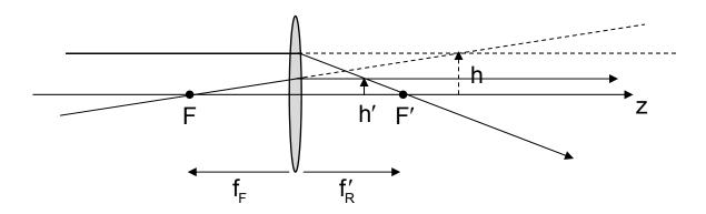
Two object rays are constructed that define the virtual object – one parallel to the axis and one through F. These rays refract to produce the real, minimized image.
