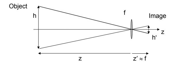
In many cases, the object/image "size" is given. It is usually considered to be centered on the optical axis with a height of  $\pm h$  or  $\pm h$ '. The height is half the size.
