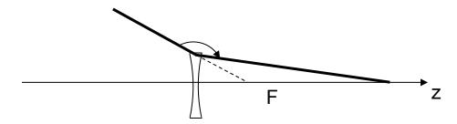
A virtual object to the right or outside the front focal point will produce a virtual image located to the left or outside the rear focal point:
