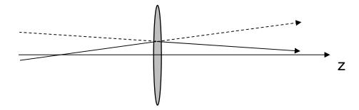
A real object is to the left of the lens; a virtual object is to the right of the lens.
