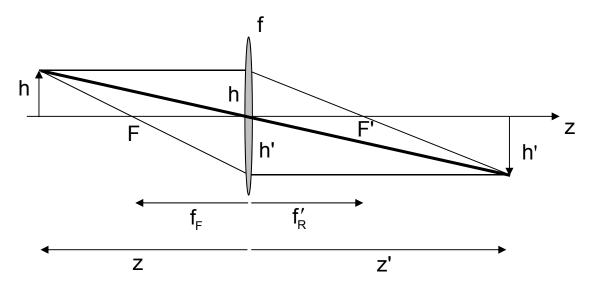
The center of the lens can be considered to be a very thin plane parallel plate. The ray is not deviated, and it displacement is zero since the plate thickness is zero for an ideal thin lens.
