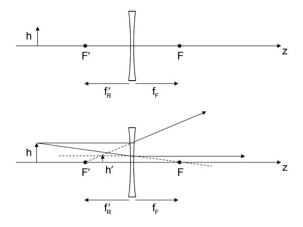
The two image space rays diverge and have a virtual crossing. A minified, erect virtual image is produced. The image is in image space.
