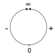
Applying this to imaging: As a real object moves through the front focal point, the image will move as a real image to positive infinity and then reappear as a virtual image coming in from negative infinity. The transition point is when the object is at the front focal point.
