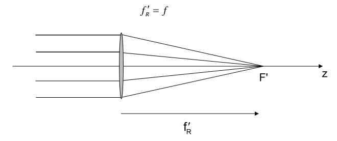
\* This discussion should actually refer to "paraxial lenses" which are perfect first-order lenses of zero thickness. Thin lenses, which also have zero thickness, may have aberrations. However, the term "thin lens" is commonly used to describe both of these idealized elements.
