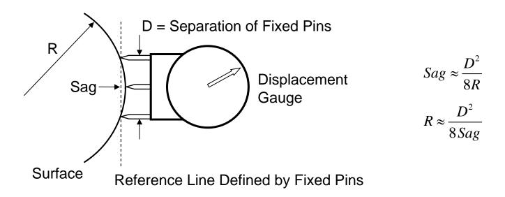
The gauge often reads in Diopters and assumes a specific index of refraction. A convex surface reads a positive power and a concave surface reads a negative power.
