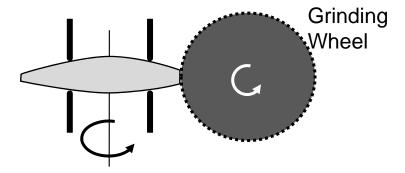
To prevent chipping of sharp edges, edge bevels are usually ground as part of this centering operation.
