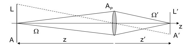
$$\Phi = L(\text{Object area})(\text{Solid angle subtended by the lens}) = LA\Omega$$
