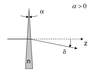
Thin prisms are used for optometric correction of strabismus (a misalignment of the axes of the eyes). The deviation is measured in prism diopters. A prism of 1 diopter deviates a beam by 1 cm at 1 m.
