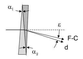
While the F and C wavelengths are corrected, a residual secondary dispersion remains. For most glass pairs, d light will be bent more than the F and C wavelengths.
