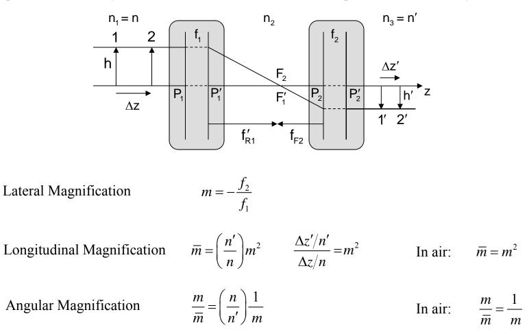
The lateral, longitudinal and angular magnifications are all constant. Equispaced planes map into equispaced planes.
