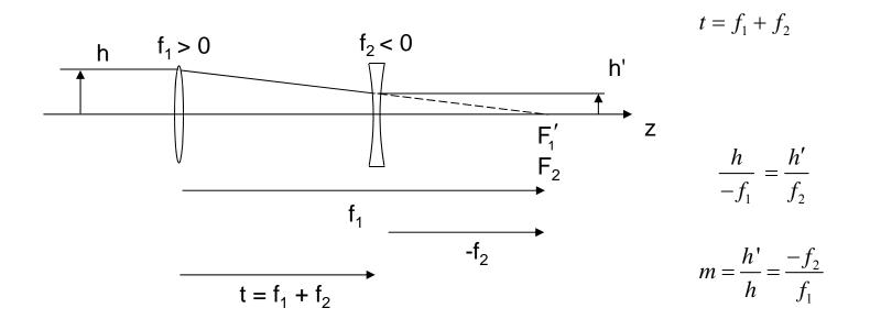
A positive system magnification is obtained in this configuration.
