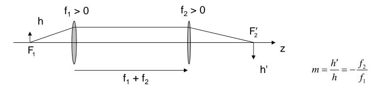
The imaging equations for focal systems do not apply to afocal systems as there are no system focal points. However, afocal systems can form images, and this will be discussed later.
