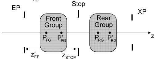
Since the Gaussian equations require the light to propagate from left to right, or equivalently that a real object is to the left of the system, the simplest conceptual solution is to flip the problem (turn the paper upside down!). The signs of the flipped distances are opposite the signs of the original distances.
