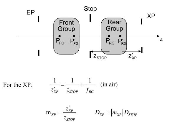
However for the EP, the stop is a real object to the right of the front group, and the Gaussian equations do not directly apply.
