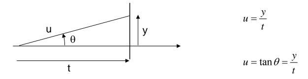
The use of ray slopes is critical for paraxial raytracing as it results in the linearity of paraxial raytracing. This is easy to see from the transfer equation:
