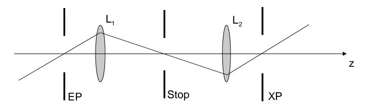
The rays are extended to the axis to locate the pupil. The EP and the XP are often virtual.
