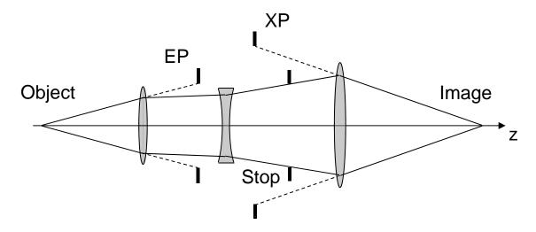
There is a stop or pupil in each optical space. The EP is in the system object space, and the XP is in the system image space. Intermediate pupils are formed in other spaces.
