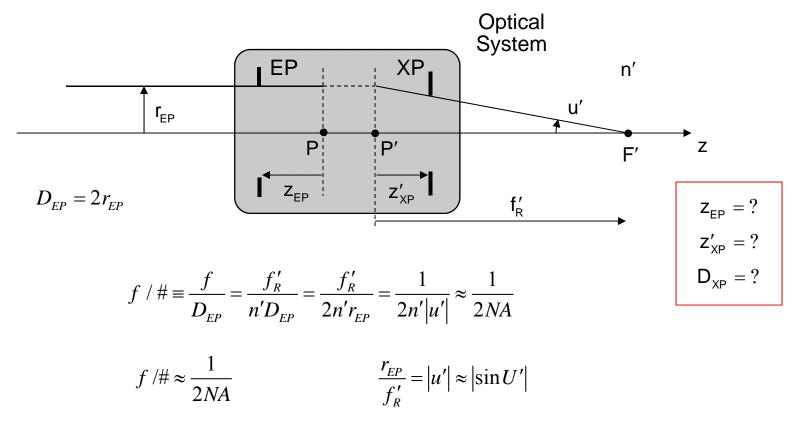
The only approximation is the small angle approximation. The image space index is expressly included in NA; it is hidden in the effective focal length for the f/#.
