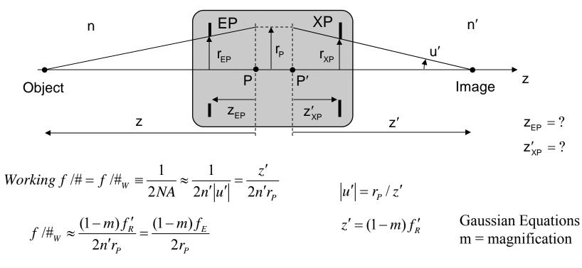
A useful relationship requires the EP size, not the ray height at P. Assuming a thin lens with the stop at the lens:  $r_P = r_{EP} = r_{XP}$
