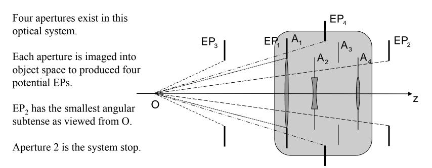
Note: All of the potential EPs are in object space.  $EP_4$  and  $EP_2$  are virtual. Since lens  $A_1$  is the first optical element, its aperture is in object space, and  $A_1$  serves as  $EP_1$ .
