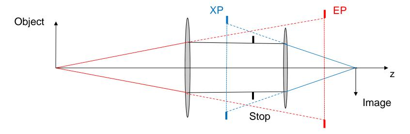
The stop and the intermediate image (not shown) define the ray bundle in the intermediate optical space.
