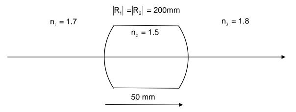
A 10 mm high object is located 100 mm to the left of the front vertex of the lens. Determine image size and the location of the image relative to the rear vertex of the lens.
