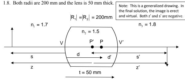
A 10 mm high object is located 100 mm to the left of the front vertex of the lens. Determine image size and the location of the image relative to the rear vertex of the lens.
