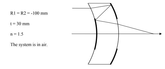
Use a paraxial raytrace to determine the back focal distance and the system focal length.
