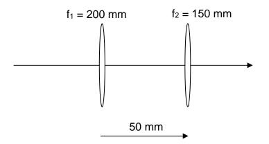
An object is placed 500 mm to the left of the first lens. The object size is  $\pm$  10 mm. Use paraxial raytrace methods to determine the system focal length and the location and size of the image.
