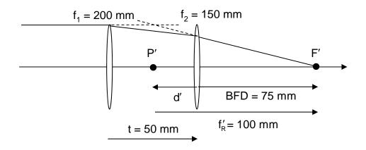
This configuration of two positive lenses places the Rear Principal Plane P' between the two lenses and is called a Petzval Objective.
