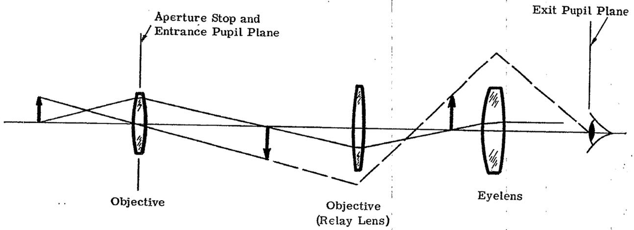
Figure 7.5 - An optical relay system or periscope.
