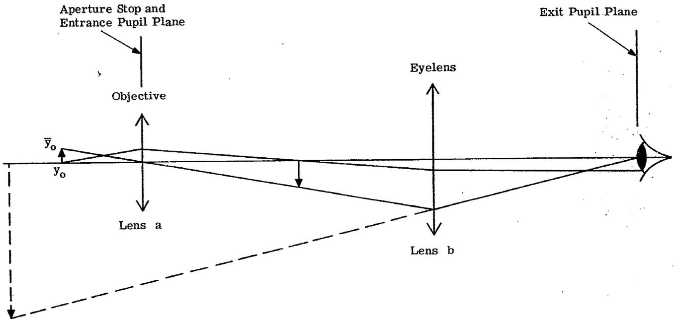
Figure 7.2 - The simple microscope. Lens (a) is the relay lens.
