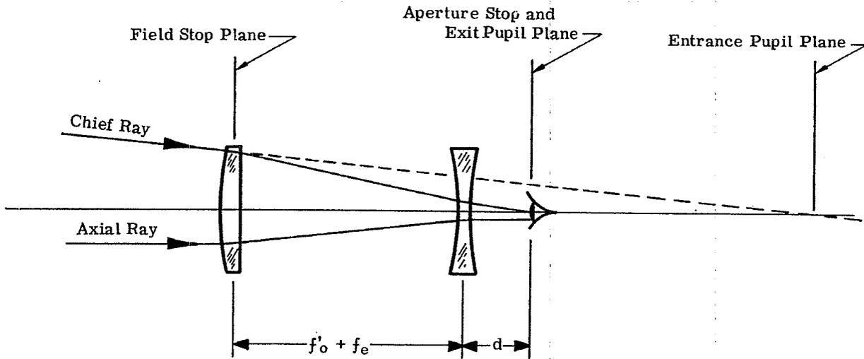
Figure 7.7 - The Galilean telescope
