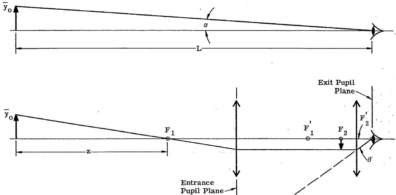
Figure 7.4. The optics of a simple telescope
