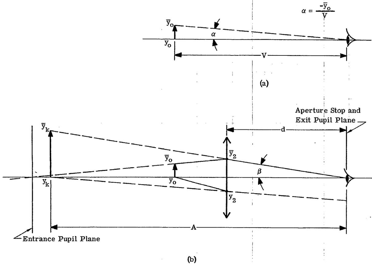
Figure 7.1 - Diagrammatic illustration of a single lens magnifier.
