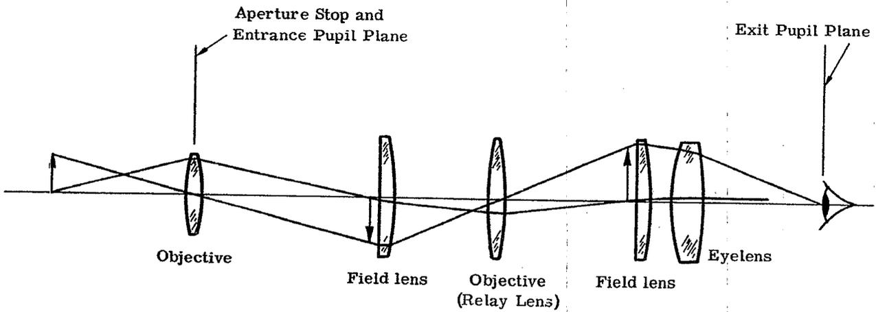
Figure 7.6 - A periscope with field lenses.
