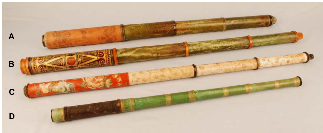
Figure 5. Paper telescopes from the early to mid-1700s: (A) Paper covered barrel and vellum covered draws, fittings made of horn. Length 840mm, barrel diameter 58mm (Leonardo Semitecolo, Venice); (B) Painted tin covered barrel and vellum covered draws, fittings made of wood. Length 810mm, barrel diameter 48mm (unsigned, German); (C) Painted paper covered barrel and vellum covered draws, fittings made of horn. Length 820mm, barrel diameter 36mm (unsigned, Italian); (D) Leather covered barrel and vellum covered draws, fittings made of horn. Length 620mm, barrel diameter 30mm (unsigned, French).
